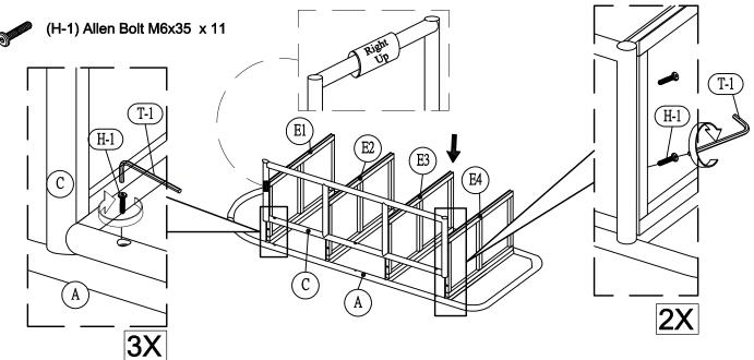
Align holes on Right Side Frame (C) with the corresponding holes on the Front Frame (A). Secure Right Side Frame (C) using Allen Bolts (H-1). Note the orientations label should be towards the top of the piece.
