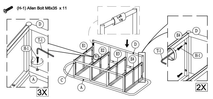
Align holes on Left Side Frame (D) with the corresponding holes on the Front Frame (A). Secure Left Side Frame (D) using Allen Bolts (H-1). Note the orientations label should be towards the top of the piece.
