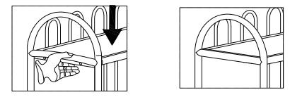
Due to the nature of the rattan material (flexible) we will sometimes need to press the component to align the holes during the assembling process
